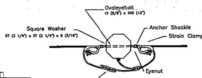
DETAIL "A", ATTACHMENT OF GROUND WIRE TO TENSION STRUCTURE
