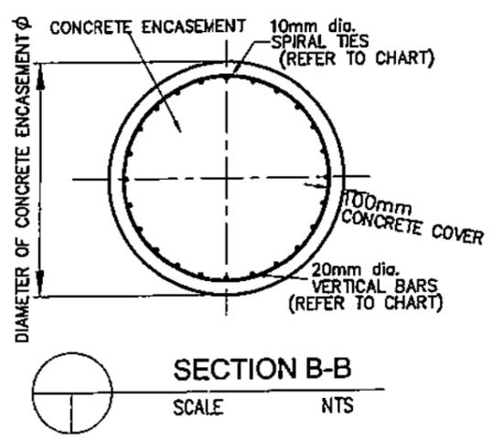
STEEL POLE CONCRETE ENCASEMENT
